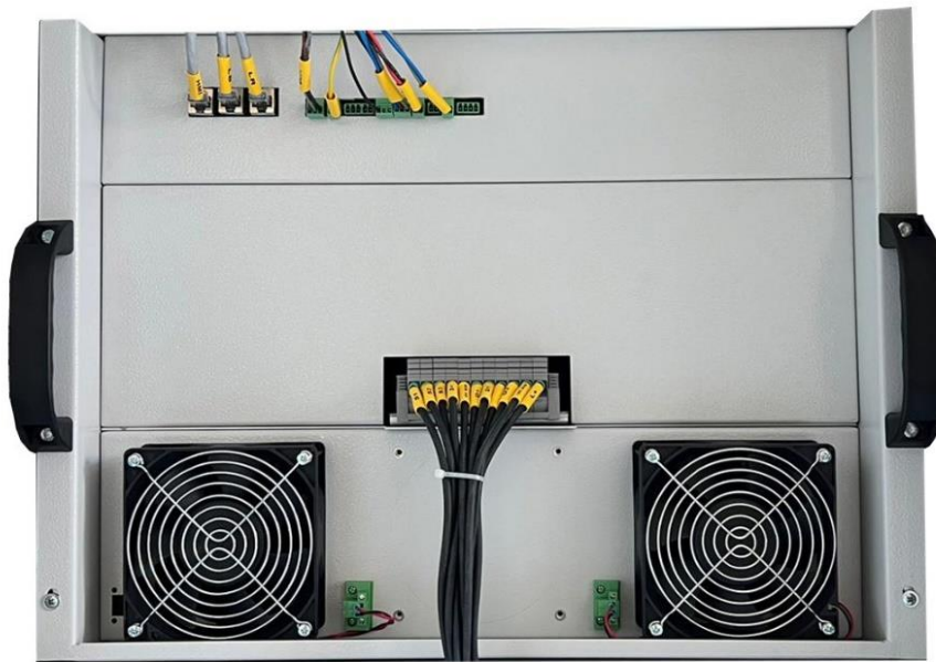
Figure 5.1. PESS RECTIFIER POWER CONTROL MODULE
