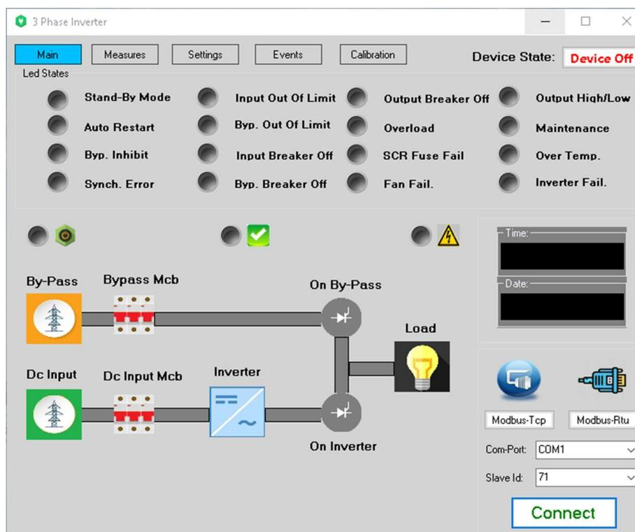
Figure 6.2. Main menu and mimic diagram of INV device
