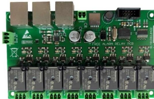
Figure 4.4. Programmable Free Alarm Relay Board
